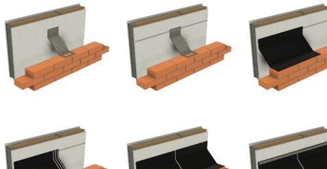
Diagram 3 - Typical preformed cavity tray corner units
