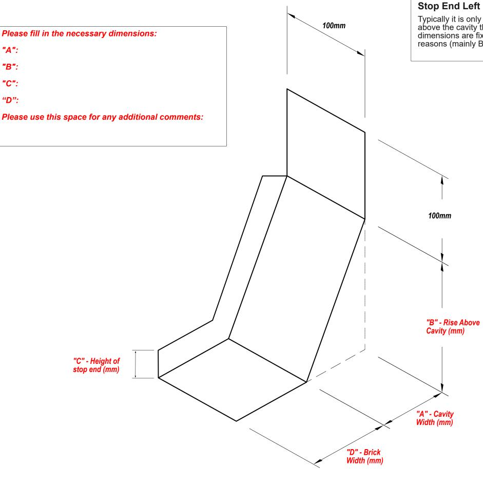
Typically it is only the cavity depth and the rise above the cavity that changes (in red). Most other dimensions are fixed for various but specific reasons (mainly BS & EN standards).
